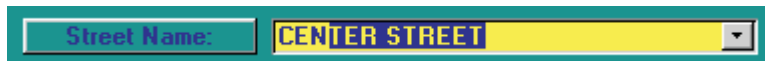
Fig. 1.5 The auto-match feature at work; the letters “C,” “E,” and “N,” have been typed in, and the system fills in a possible match, spelling “Center Street.”
