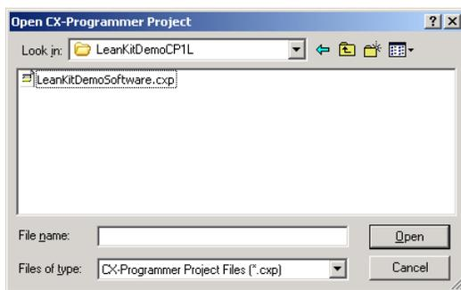
Connect the USB programming cable (CP1W-CN221) between your PC's USB port and the CP1L PLC 'Peripheral' (USB) port, located behind the flap on the left-hand side. If this is the first time you have connected to a PLC, you will see this screen...
