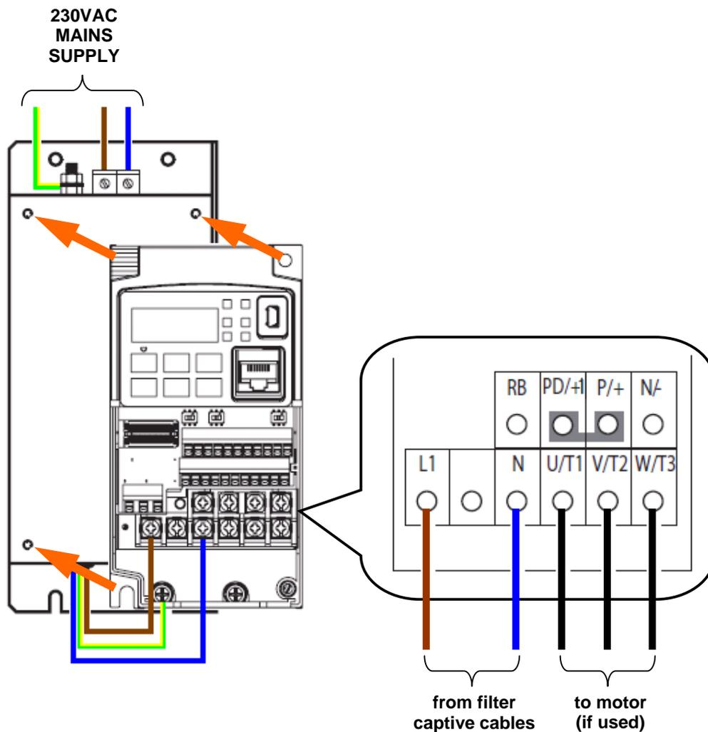
1. Attach the MX2 inverter to the filter using the M4 screws (4 off) supplied with the filter.
