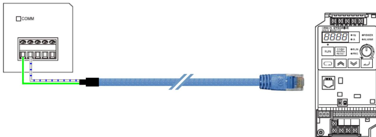
1. Insert the RJ45 connector end into the front of the JX inverter (located behind the rubber flap)
