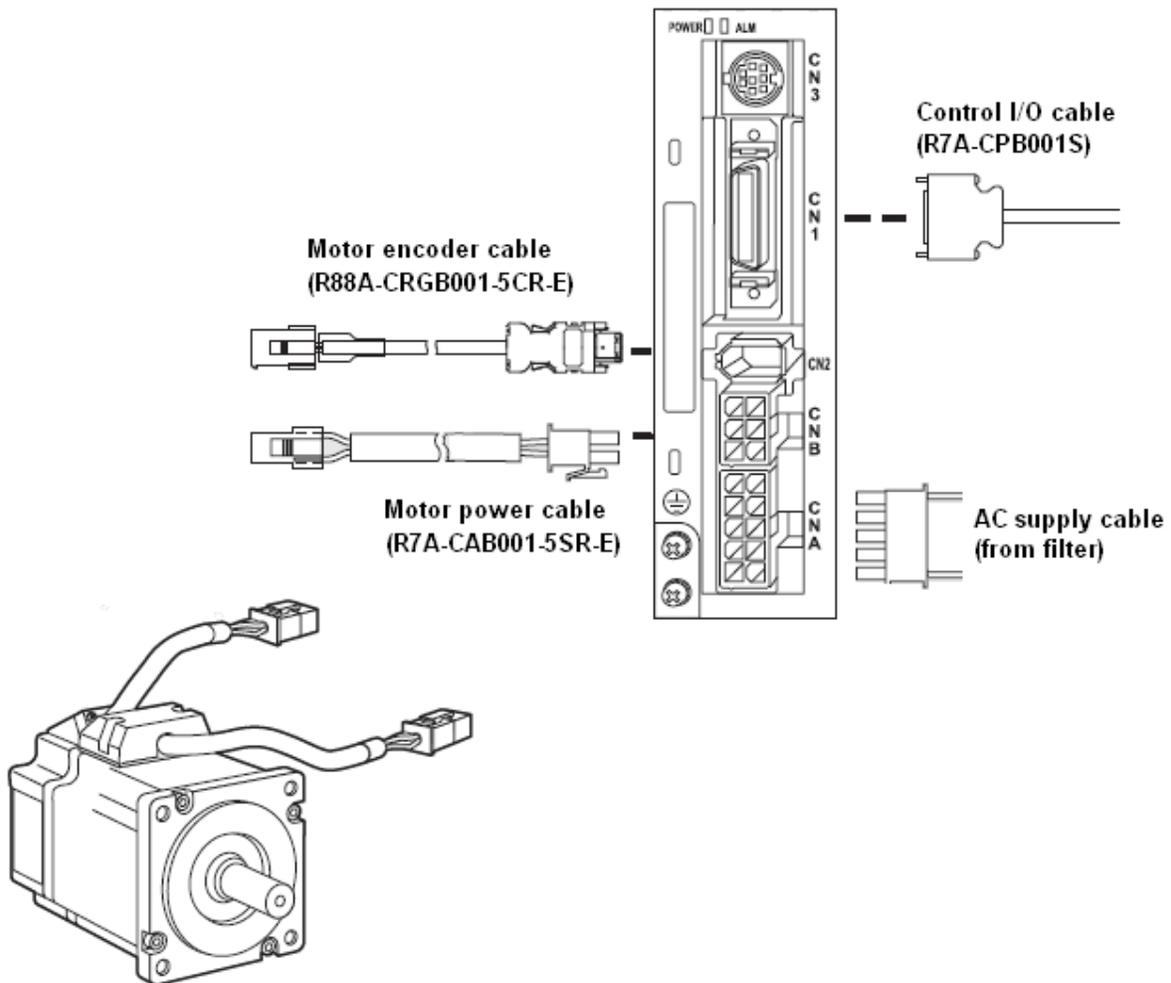
5. Attach the control I/O cable (R7A-CPB001S) into terminal 'CN1' of the servo amplifier and secure the retaining screws.
