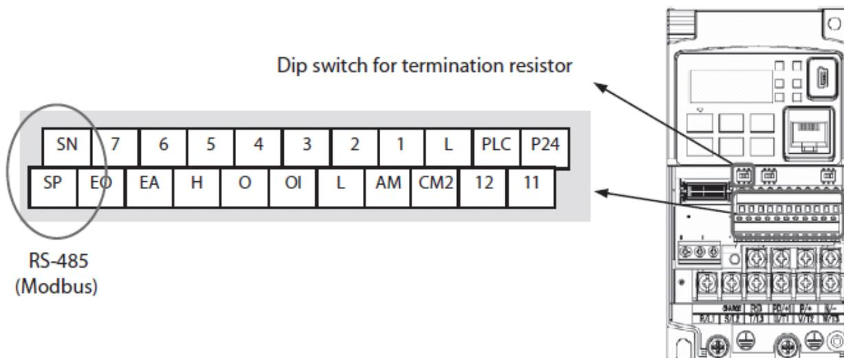
Up to 31 inverters may be connected to a MODBUS 'master' (in this case, the CP1L PLC), using unshielded, twisted-pair cable is used to 'daisy chain' them together. Suitable cable is Belden 9502 or equivalent.
