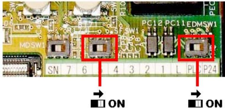
Turning the middle switch to the ON position sets digital inputs 3 and 4 to be used as normally-closed safety inputs. This action automatically forces drive parameters C003=77 and C004=78 to define the use of these safety inputs.
