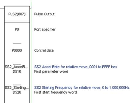
The 'PLS2' instruction sends a number of pulses from a transistor output at a set frequency.
