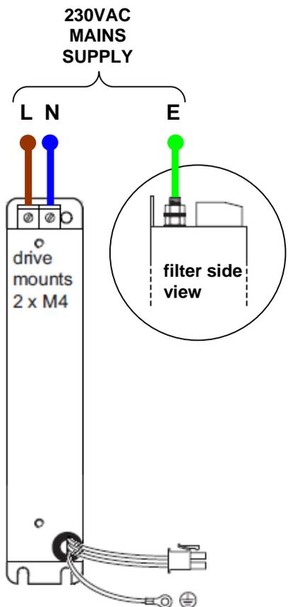
1. Connect a 230VAC supply to the filter, as shown in the diagram above, ensuring that an earth connection is made to the M4 stud behind the terminal block.
