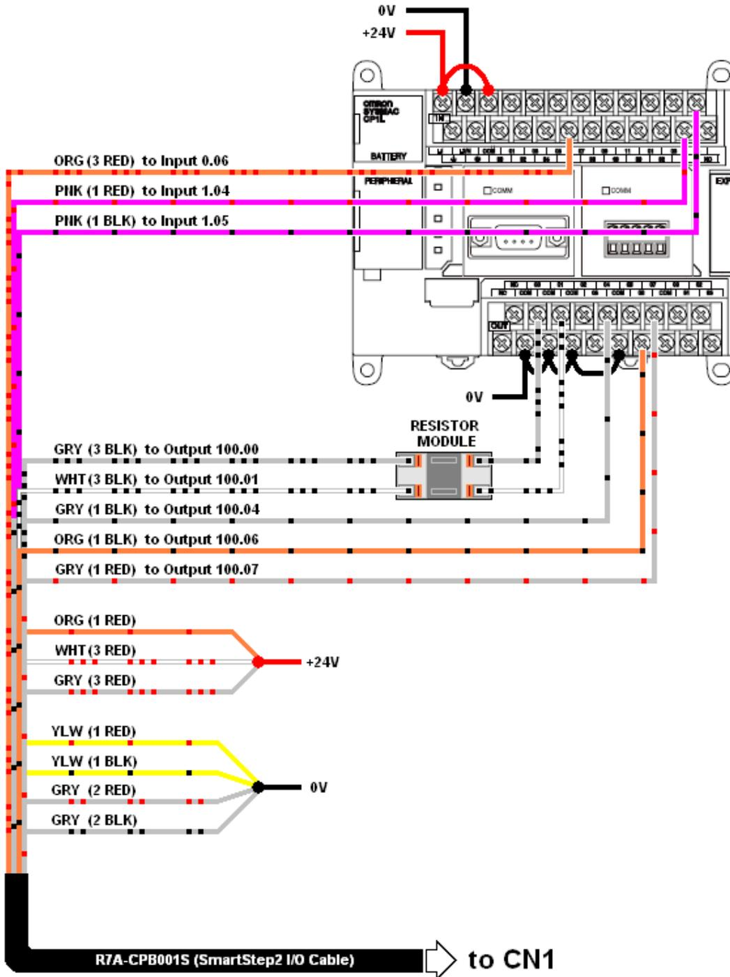
SmartStep2 servo amplifier to PLC wiring;
