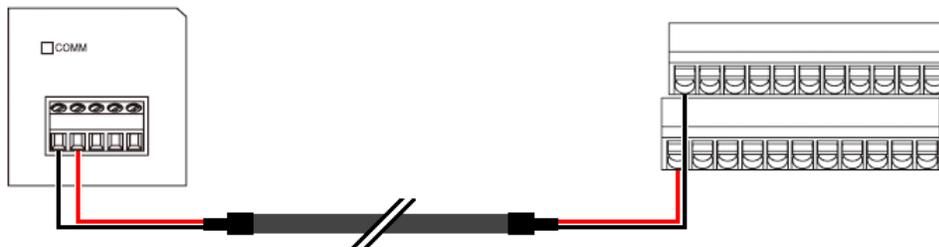
1. Using the supplied cable, connect the black wire to the first screw terminal of the CP1W-CIF11 module (marked RDA-) and the red wire to the second screw terminal (marked RDB+).
