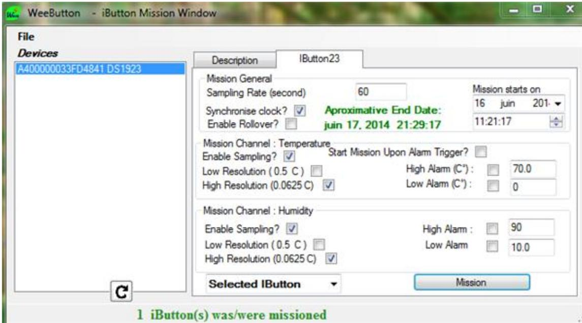
You will then see at the bottom of the window: **1 iButton(s) was/were missioned**. This means that the mission launch was successful. Note that whenever a mission is programmed, all data from a previous mission is lost, and all memory is set available for the new mission. You are now ready to deploy!
