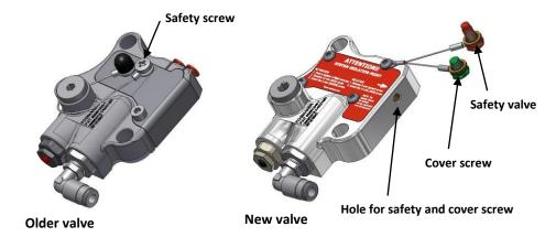
The release valve has a transport safety called "safety screw"; the safety screw shall be removed when the system is active. There are two types of release valves. One older version with the safety screw fitted from above, remove to activate the system.
