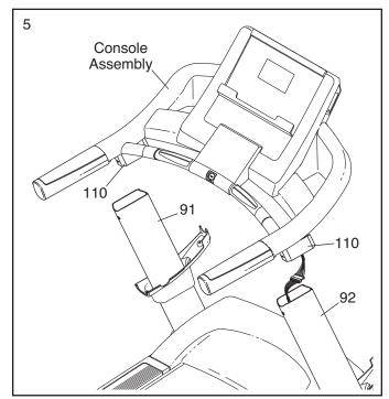
Partially tighten three 3/8" x 1 1/4" Patch Bolts
