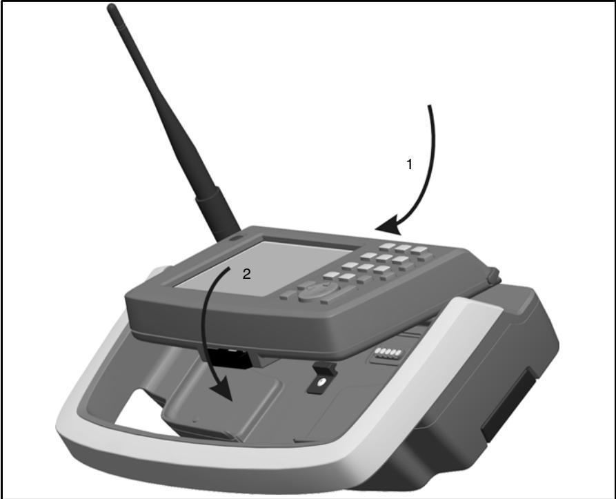
Figure 7.68 Attach Trimble CU to Trimble Robotic Holder
