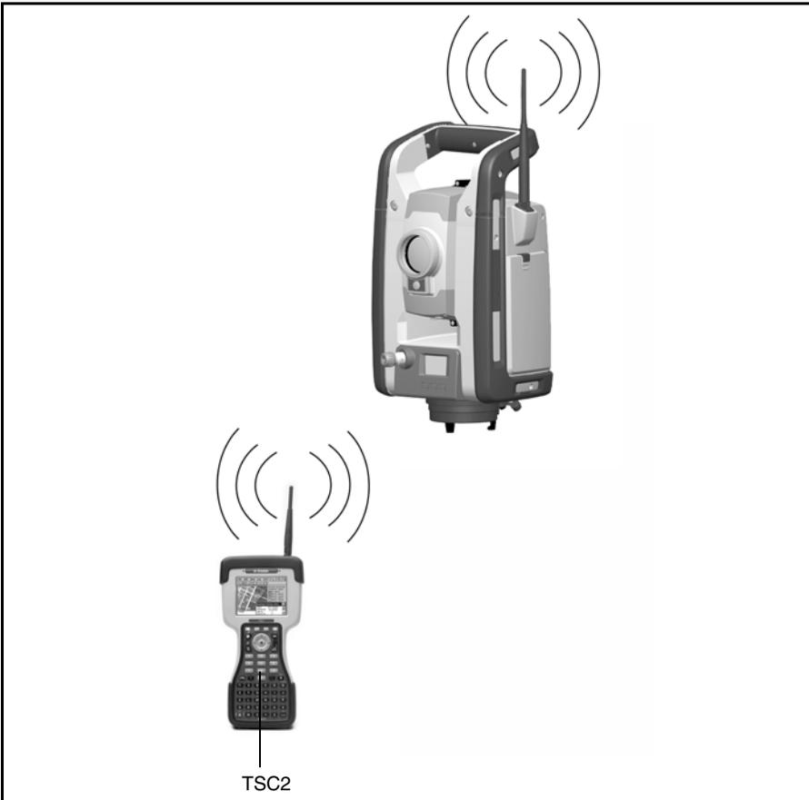
Figure 4.40 TSC2 connected to the SPS Series Total Station using the inbuilt radio for robotic measurements.
