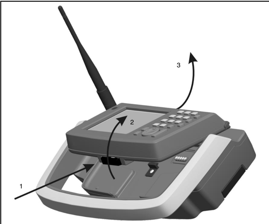
Figure 7.69 Detach Trimble CU from Trimble Robotic Holder
