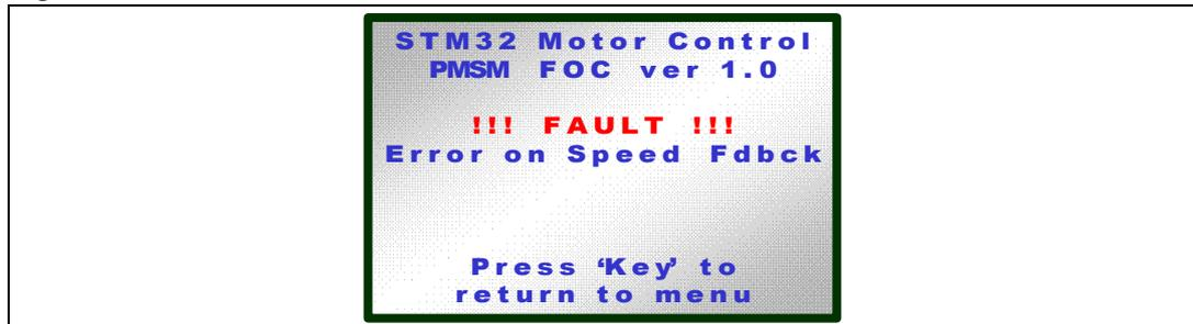
"Press 'Key' to return to menu" is displayed only if the cause of the fault is no longer present. Pressing the 'Key' button causes the main state machine to switch from FAULT to IDLE state. Six different fault sources are monitored during operation. Refer to the UM0492 STM32 sensorless PMSM field-oriented control software library user manual for more implementation details.
