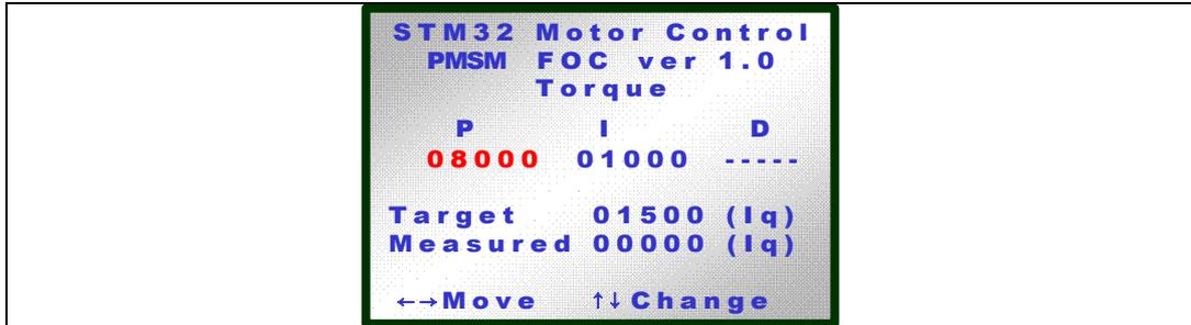
This regulator can be tuned in the same way as the speed regulator. Pushing the joystick twice to the right enters the Flux regulator settings screen.
