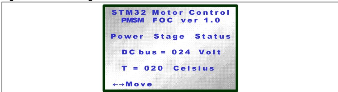
Pushing the joystick on the right enters the Sensorless control settings screen, to modify the rotor position observer gains K1 and K2, as well as the PLL gains (this PLL provides the speed feedback for the speed regulator, using the rotor angle computed by the observer).
