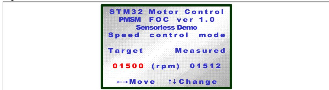
When the motor is running, the LCD indicates the target as well as the measured speed. Pressing the joystick up/down increases (or decreases) the speed set point respectively.
