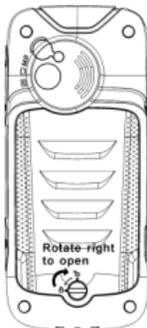
2. Open the battery cover using the thumb notches on the bottom on the cover.
