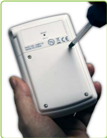
Using a cross head or flat bladed screwdriver, remove the Sender Unit battery compartment cover and insert 3 AA batteries. Press and hold the RESET button located on the rear of the Transmitter.
