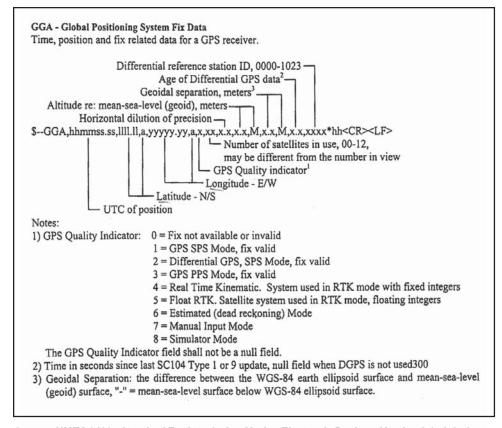
Source: NMEA 0183 - Standard For Interfacing Marine Electronic Devices, Version 3.0, July 1, 2000.
