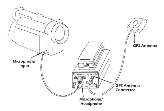
Shown is the simplest configuration for recording video with VMS 300.
