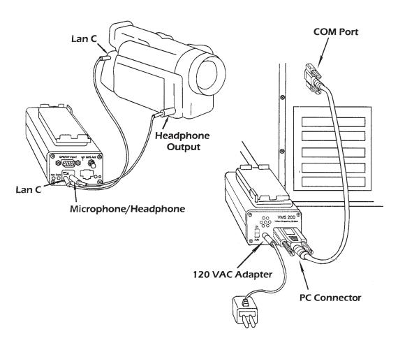
Both front and back views of a single VMS300 hardware unit are shown in this setup diagram. You may also have a video capture card connection between the camera and computer, and you may have your computer sound card connected to the camera as well. These options depend on whether you want to capture video and view real time video on screen, or capture sound files. Follow manufacturer's instructions for your device.
