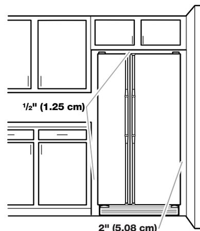
**NOTE:** Do not install the refrigerator near an oven, radiator, or other heat source, nor in a location where the temperature will fall below 55°F (13°C).
