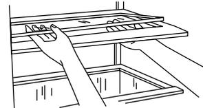
3. Replace back of meat drawer cover frame into supports on side walls of the refrigerator and lower the front of the cover frame into place.
