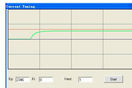
Figure 23: Kp=2346, Ki=0 (poor performances)
