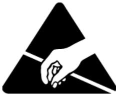
The ESD warning label appears on packages and storage bags that contain static-sensitive products and components.
