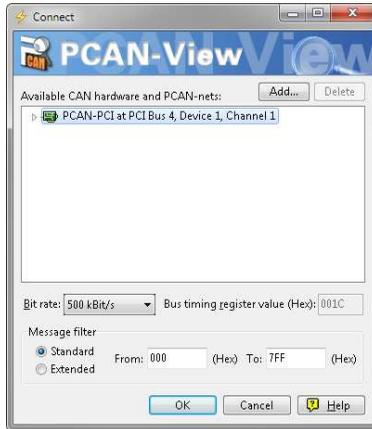
Figure 6: Selection of the CAN hardware and parameters
