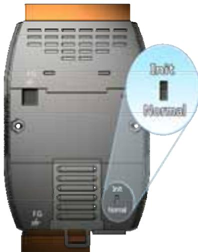
Make sure the switch placed in the "Init" position.
