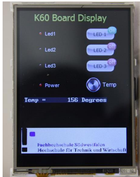
Figure 49 - LCD module simulation for touch and data display
