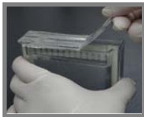
Remove the top sealing film
