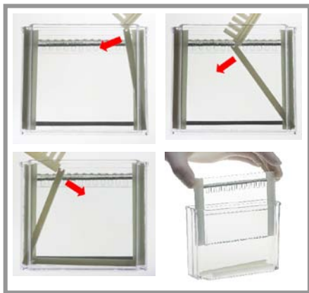
Release the gel sandwich
