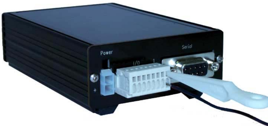
Figure 10: Wago Connector Wire Insertion
