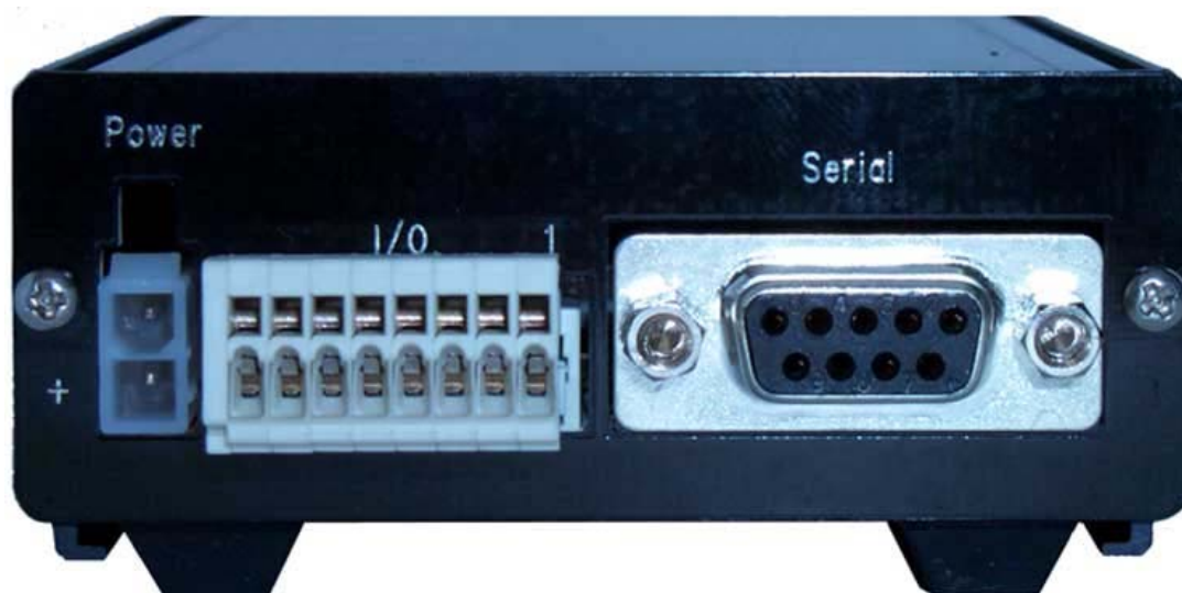
Figure 2: Rear view of GSM1208 Spider SA-G modem.
