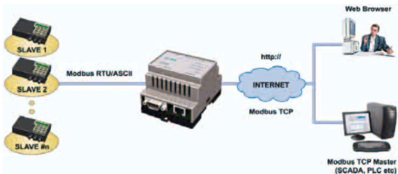
The protocol converter Modbus TCP/RTU supports an RS-232 connection through a 9-pole DSUB and RS-232 or RS-485 through the screw terminals. It also supports 10/100Mbps Ethernet through a standard Ethernet connector (RJ-45). It can be configured via a user-friendly web-interface or by using the Config utility.
