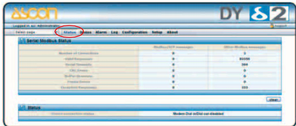
**Number of connections** - Indicates the number of open connections to a Modbus TCP master. Internal queries indicate number of pending queries from WebPages + the internal connection from (Alarm/Log) application.
