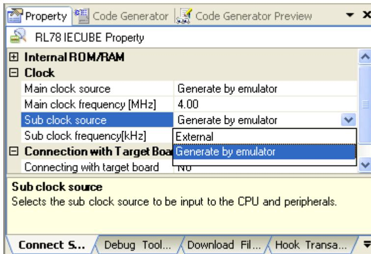
**Note** This setting is not possible when TARGET LED is not lit.
