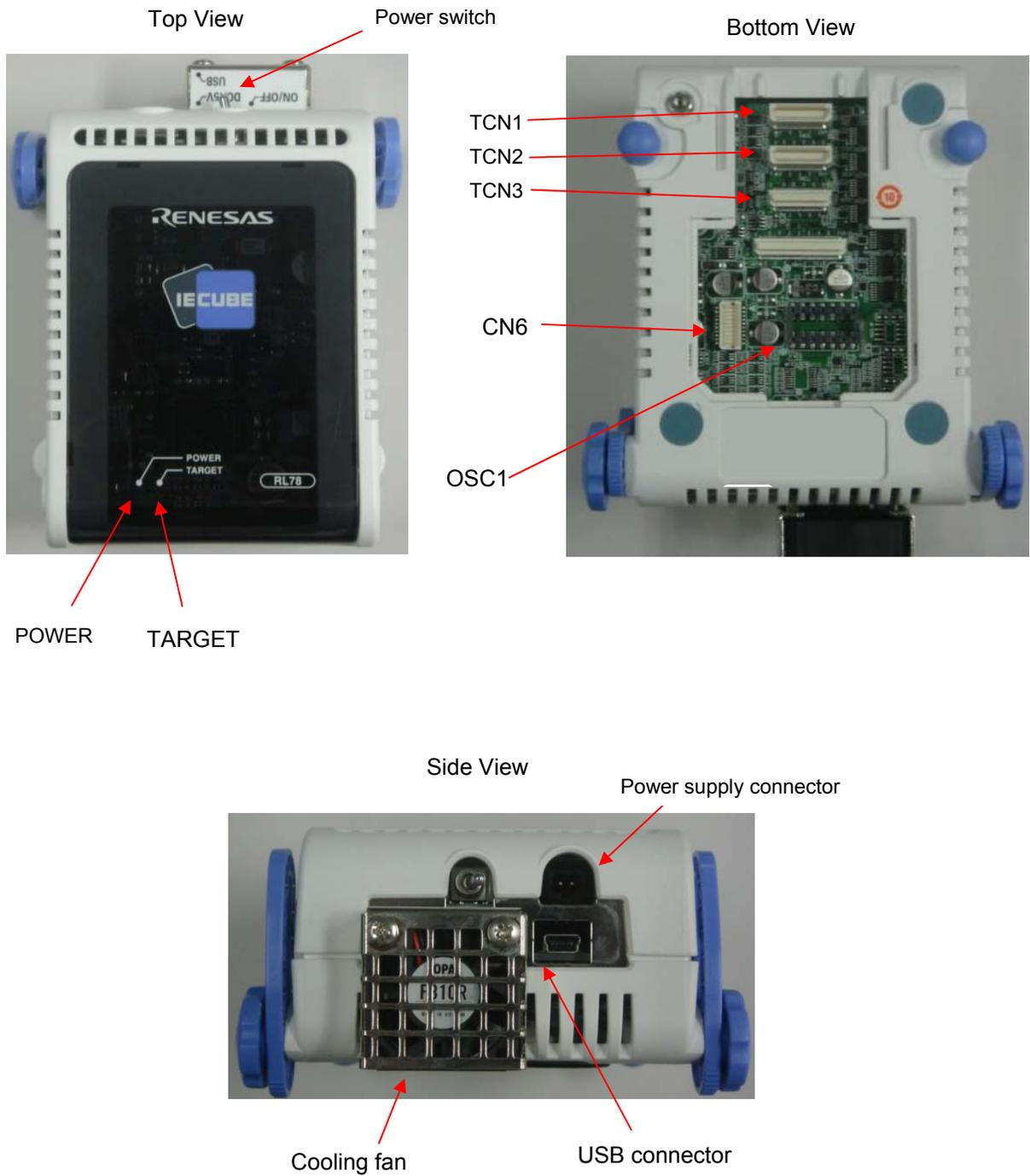
Figure 1-1. Names of Parts of QB-RL78F12
