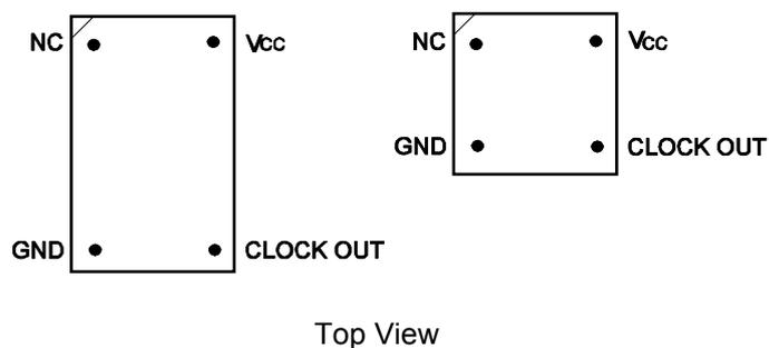
Figure 2-3. Mapping of Oscillator to Socket
