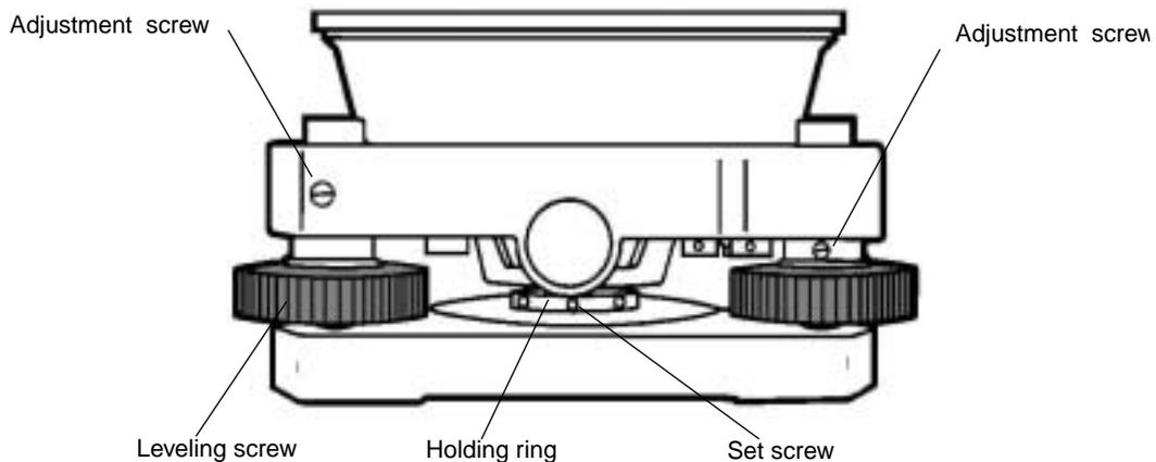
**17.3.1 Checking /Adjusting the Plate Level**
