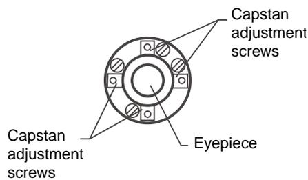
Note: 1 First, loosen the capstan adjustment screw on the side to which the vertical cross-hair line must be moved. Then tighten the adjustment screw on the opposite side by an equal amount which will leave the tension of the adjustment screws unchanged. Revolve in the counterclockwise direction to loosen and in the clockwise direction to tighten, but revolve as little as possible.
