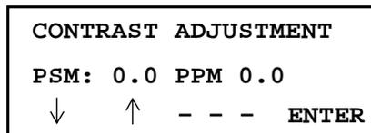
This enables you to adjust the brightness by pressing the [F1]( ↓ ) or [F2]( ↑ ) key. To memorize the setting value after powering off, press [F4](ENTER) key.
