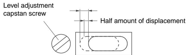
**17.3.2 Checking /Adjusting the Circular Level**
