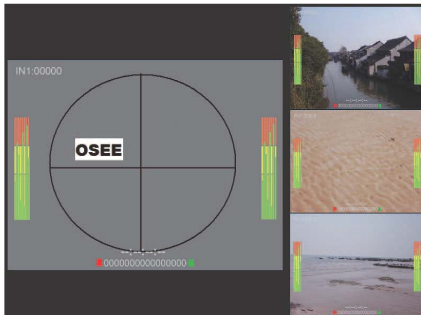
One-big and with three-small screen, full 16-channel audio meter
