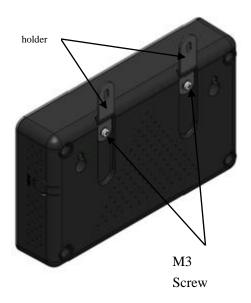
• Fix the ECU on the frame with screws and keep it away from other heat-generating devices.
