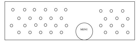
You can access the ECU LCD panel menu by pressing and holding the Menu button; after two seconds you will enter the ECU menu. Continue holding the button, and menu items will appear in the following order:
