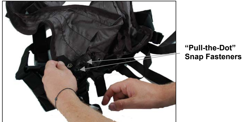
Figure 36. Step e. Webbing and Snap Attachment System at the Lobe
