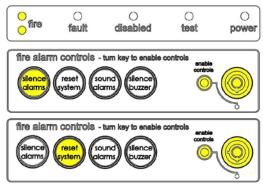
The red 'FIRE' LED will illuminate. The fire alarms and the internal buzzer will operate as programmed. Take appropriate action as defined by the emergency plan for the premises.
