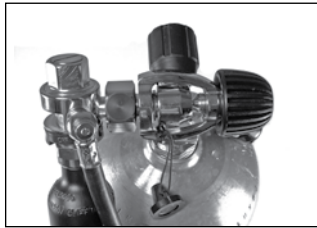
Figure 4 - Filling the H.A.B.D.
