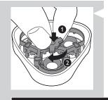
5 Put the retaining frame back into the shaving unit, push it down (1) and turn the wheel clockwise (2).
