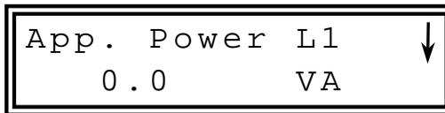
Figure 5-5. **Apparent Power Screen**
