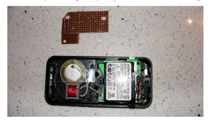
Unit wired ready to plug in the transceiver. Note the six ferrite sleeves on the audio cable to the TRX.
