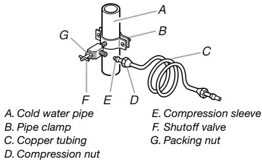
6. Fasten the shutoff valve to the cold water pipe with the pipe clamp. Be sure the outlet end is solidly in the ¼" (6.35 mm) drilled hole in the water pipe and that the washer is under the pipe clamp. Tighten the packing nut. Tighten the pipe clamp screws slowly and evenly so washer makes a watertight seal. Do not overtighten or you may crush the copper tubing.
