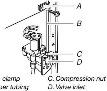
6. The ice maker is equipped with a built-in water strainer. If your water conditions require a second water strainer, install it in the ¼" (6.35 mm) water line at either tube connection. Obtain a water strainer from your nearest appliance dealer.
