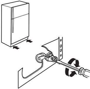
3. Open both doors again and check to make sure that they close as easily as you like. If not, tilt the refrigerator slightly more to the rear by turning both leveling screws to the right. It may take several more turns, and you should turn both leveling screws the same amount.
