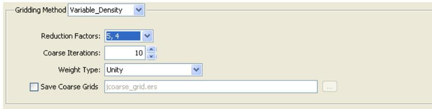
This method was designed especially for gravity data acquired at variable sampling densities, over the region you wish to create a gridded representation of the field. The basic intent of the method, is to estimate various wavelength contents optimally, and to combine them into one, final grid that has the best assemblage of observed wavelengths from the datasets provided.
