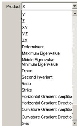
You can choose to produce either a range of one-band scalar grids, or a full tensor grid.
