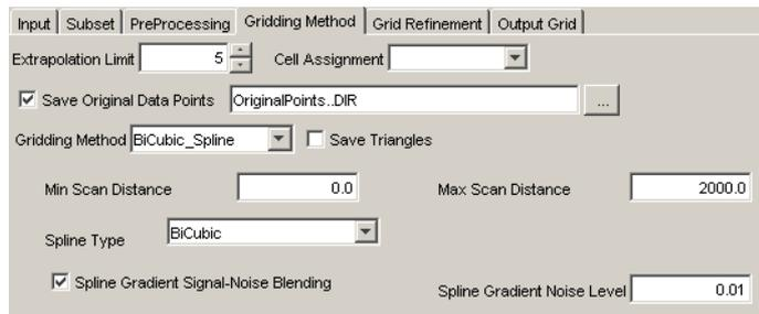
While using this method of calculating values for interpolated cells, INTREPID creates a located line structure that is closely related to the columns and rows of the grid being created. There are three stages of gridding with this method.
