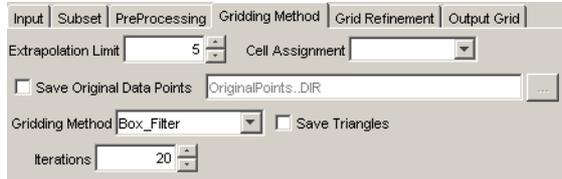
The Box Filter assumes that the original data points are at the cell centroids. It does not take account of the actual position of data points within the cell (i.e., it has no 'honour original points' process) and therefore may not be as accurate as other methods.
