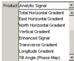
You can choose the following derived grid products. The illustration shows the **Product** drop-down list in the **Output grid** tab (see [Output Grid tab](#)).
