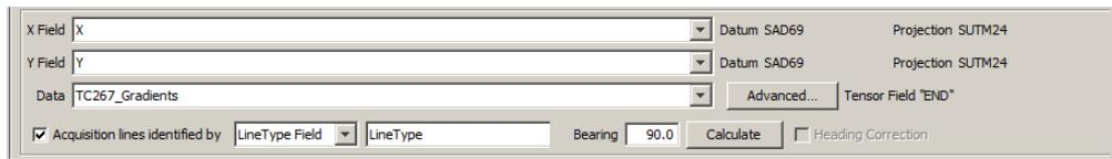
For multiband datasets the Advanced button changes to a band selector with the total number of bands available shown to the right
