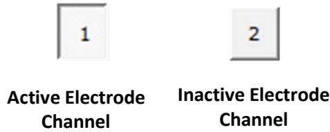
Figure 3-7: Status of Manual Mode Electrode Channels
