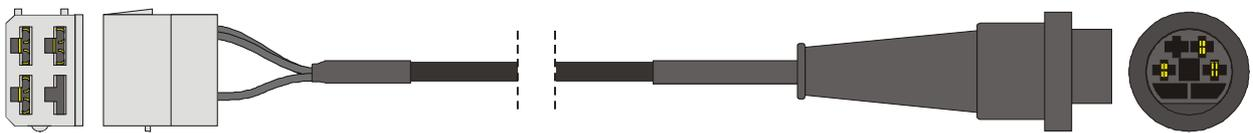
02.35 Measurement cable for checking the "4" sender - tachograph 1314
