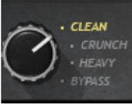
**Guitar Mode** toggles between guitar modes. In Bypass, mode-specific processing is inactive when Re-Amplify is Off; when Re-Amplify is On, Bypass also turns off the modeled guitar amp.
