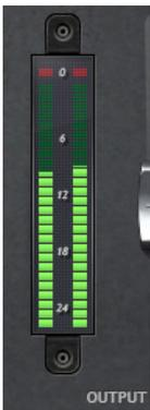
**Output Meter** displays output signal peak level.
