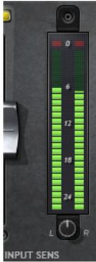
**Input Meter** displays input signal peak level.
