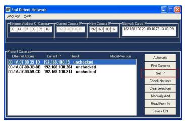
Click Set IP to set the IP address. To configure additional information for the camera, go to the camera's web page.
