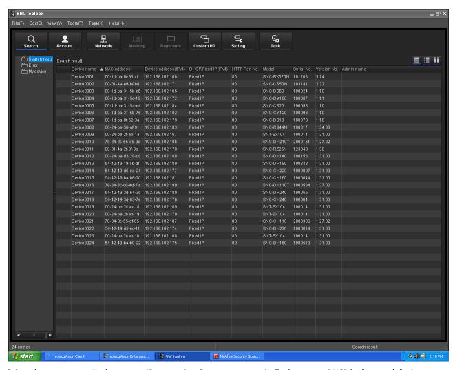
Select the camera to edit the camera IP properties. Sony cameras typically do not use DHCP by factory default, you must manually assign the camera an IP address. Enter an IP address that is not used by any other device on your local network, ensuring that the first three numbers match the first three numbers of your IVTVision Server's IP address. Set the subnet to 255.255.255.0, leave the HTTP port at 80, enter the camera's Administrator name and password, and click Apply.
