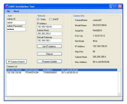
To change the IP address of the selected camera, select Static in the Network area. Enter the IP address and default gateway, and then click Set IP Address.
