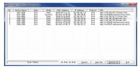
Samsung cameras on the network are listed. Click Search to update the list. To change the network settings for a camera, highlight a camera and select **Manual Set**. This opens the following window:
