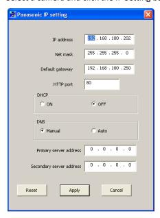
Panasonic cameras typically do not use DHCP by factory default, you must manually assign the camera an IP address. Enter an IP address that is not used by any other device on your local network, ensuring that the first three numbers match the first three numbers of your IVTVision Server's IP address. Set the net mask to 255.255.255.0, leave the HTTP port at 80, enter the camera's Administrator name and password, and click Apply.
