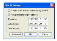
Enter the IP address, subnet mask, and default router. Click OK to apply the IP address.
