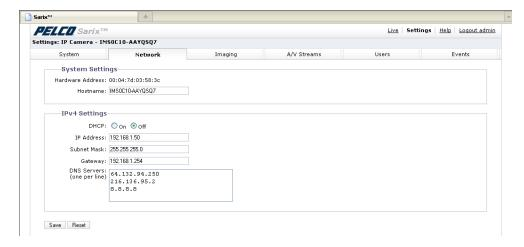
To change the IP address, select Off next to DHCP and type the address. Click Save when finished.
