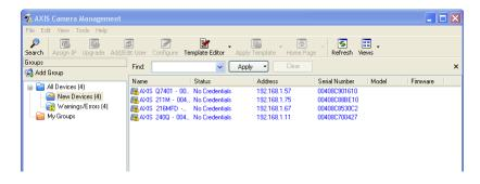
AXIS cameras on the network are listed. Right-click a camera and select Enter Device Credentials....
