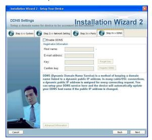
Do not select Enable DDNS unless you are planning to put this camera on the Internet. This is not recommended. Click Next to complete the configuration.
