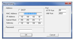
Enter the IP address, subnet mask, and default gateway. HTTP Port is used to access the camera in a web browser (the default is 80). VNP Port is used to control the video signal transfer (the default is 4520). Leave the Password box blank to keep the default password. Click OK to apply the new settings.
