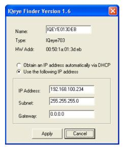
IQinVision cameras typically do not use DHCP by factory default, you must manually assign the camera an IP address. Enter an IP address that is not used by any other device on your local network, ensuring that the first three numbers match the first three numbers of your IVTVision Server's IP address. Set the subnet to 255.255.255.0 and click Apply.
