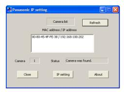
Select a camera and click the IP Setting button to view and edit the camera's IP properties.
