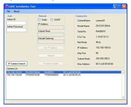
All Ganz IP cameras on the local subnet are listed in the Camera List section. Select a camera to display information in the Camera Info area.
