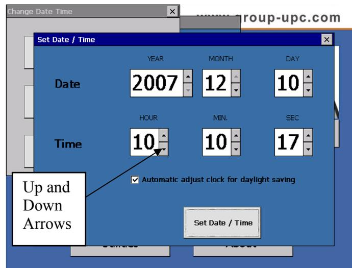
Use the up and down arrows to change the Date and Time. After the correct date and time are entered touch the *Set Date / Time* button. The new Date and Time will then be saved. Touch the x in the upper right hand to close the window.
