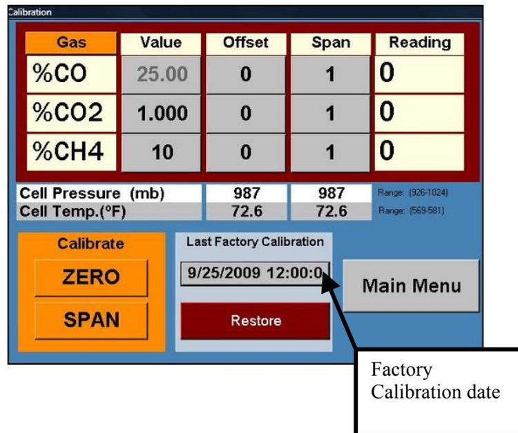
When you send your analyzer into Furnace Control Corp. for calibration, the calibration data, and the factory calibration date are entered and stored in the analyzer's memory by the use of a password.
