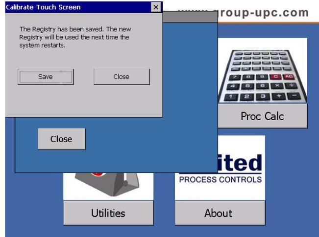
Touch *Close* and the touch screen calibration will be saved. The new setting will apply the next time the unit is turned back on.
