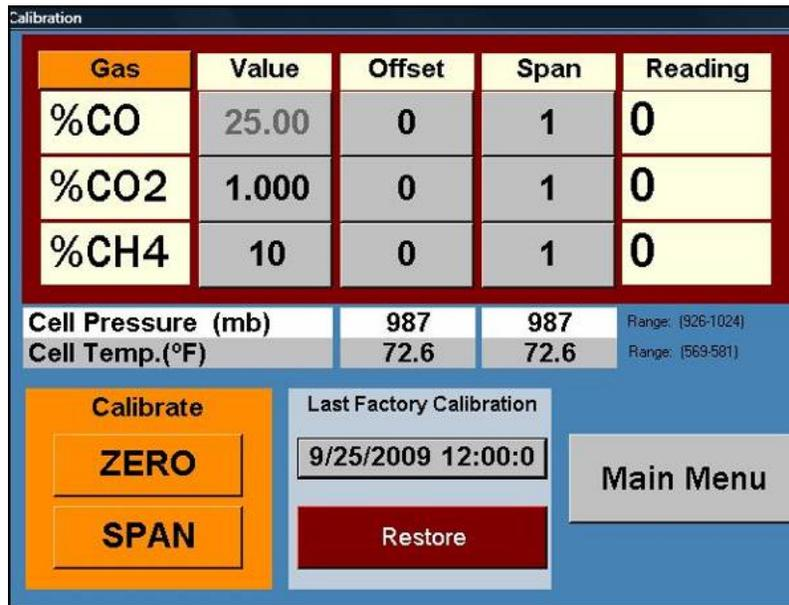
Once the unit has counted up to 120 the calibration is complete. You can now return to the *I/R Gas Values* screen. The instrument should read the values in the bottle within 2% of the cell range. (I.e. 30% CO should be +/- .6% CO.)
