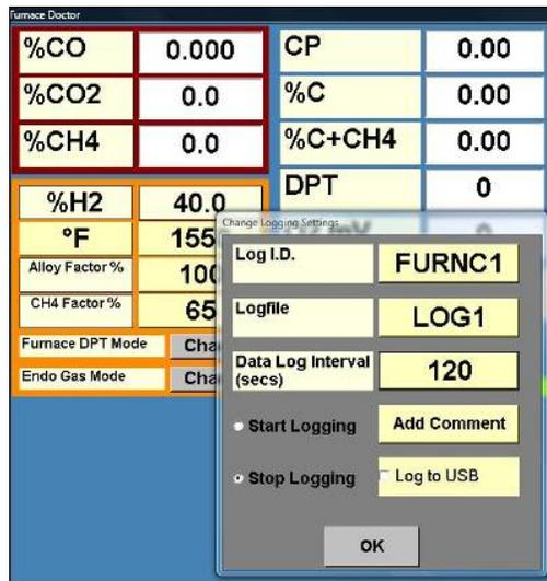
A window pops up stating *Please insert an USB memory stick*. Insert the USB stick and touch OK to start data logging.
