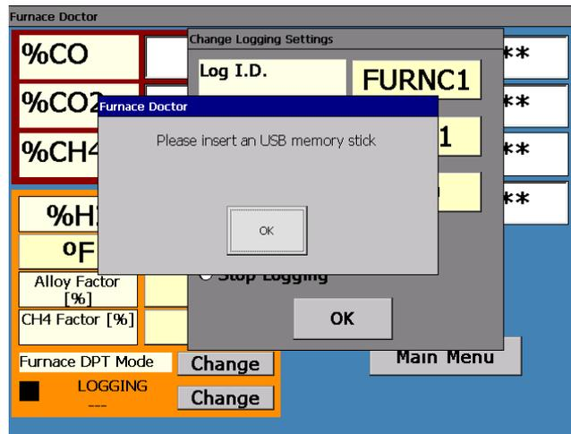
After Touching OK the text next to the *Change* button will state *Logging: ON* and will display the *logfile* name in green.
