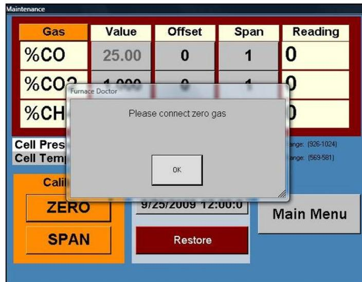
After nitrogen has been connected and there is adequate flow press *OK* to start the calibration.
