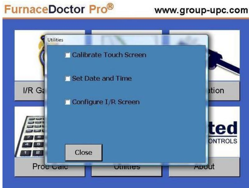
**Calibrate Touch** – Allows you to calibrate the touch positions on the screen by locating a target for you to touch at various positions on the screen.
