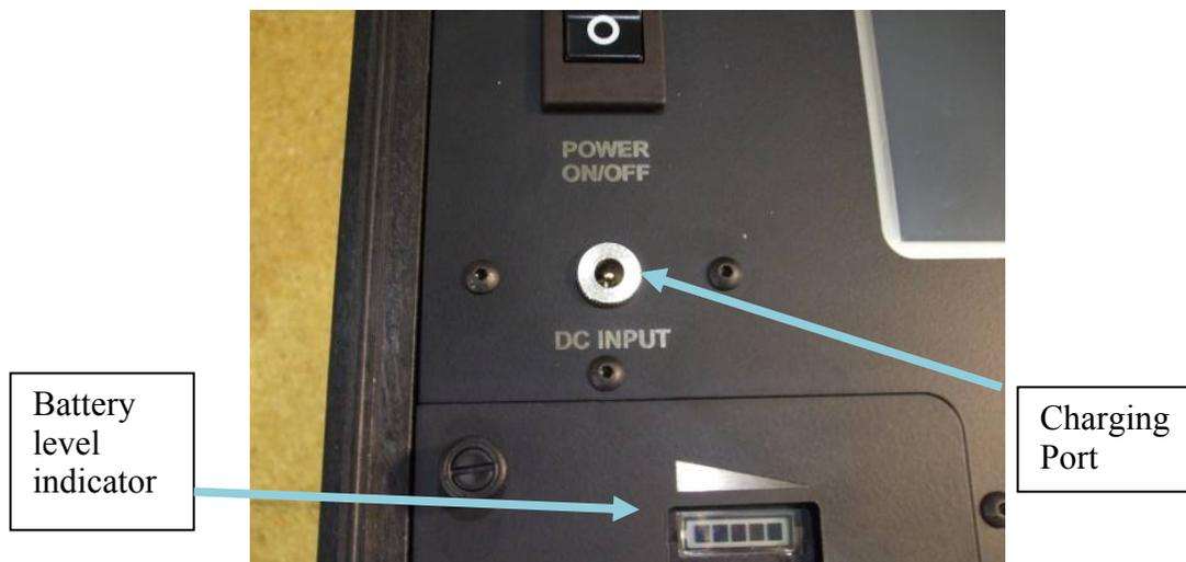
***Note: Unit is designed to operate with a charged battery or with the A/C adaptor. Using the charger as an AC adapter will not allow the battery to charge as quickly as it would otherwise. It is a best practice to connect the charger with the unit's power off and fully charge the battery. The unit will not operate with the battery removed.***
