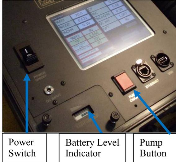
The LCD display will illuminate, and the internal pump will start after pump button is depressed. Manually inputted fields are in yellow, live and calculated fields are in white. Buttons are grey.
