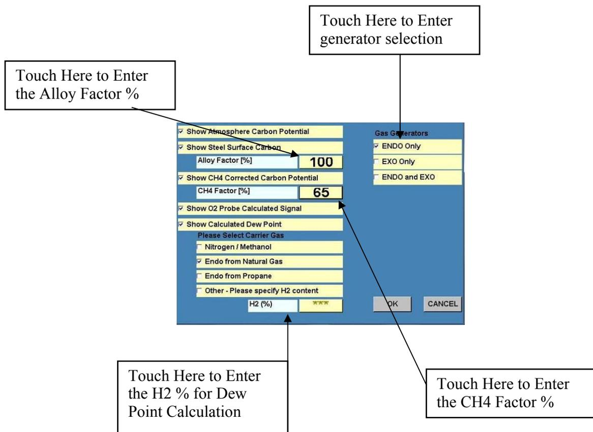
To Enter the *Alloy Factor %*, *CH4 Factor %*, and the *H2 %* for Dew Point and carbon potential calculations touch the corresponding box. An alpha numeric keyboard will appear to enter the value. Touch **OK** when done.
