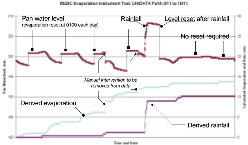
The derived evaporation and rainfall data is the accumulated total since the logger was last reset. It may contain corrupting events if there has been any artificial water level changes. There are two shown in the above example. These can be removed by editing the data in a spreadsheet or with one of a range of commercial editing systems.
