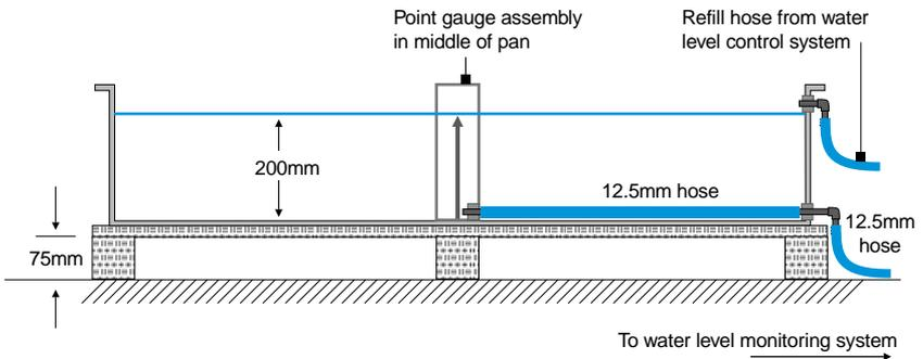
Rest the pan centrally on the pallet. Rotate it to orient the hole in the pan toward the location of the stillwell assembly. Assemble the hose fittings through the hole at the bottom of the sidewall of the pan. Seal the joints with a smear of silicon. The assembled fitting has a hose barb on each side of the tank wall.
