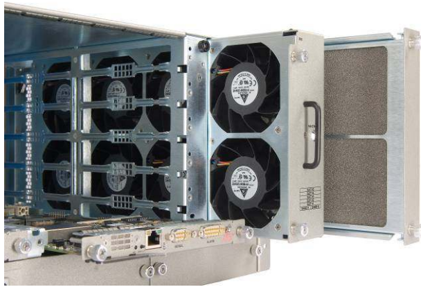
Figure 21 – Extracting a Fan Tray
