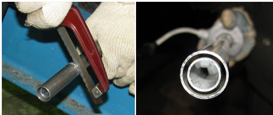
Figure 12 — DUT-E measuring probe cutting
