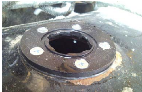
Figure 8 — Mounting plate fastened to the standard sensor flange
