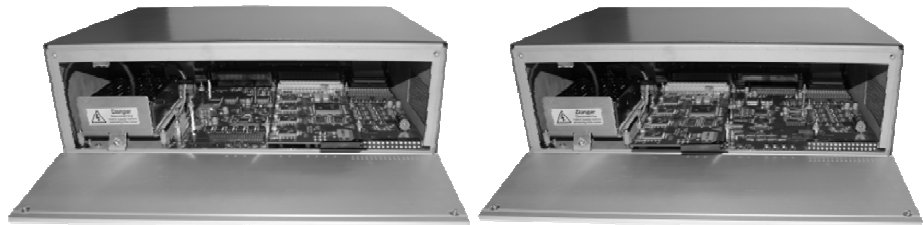
Fig. 9 Fitting one quad card
