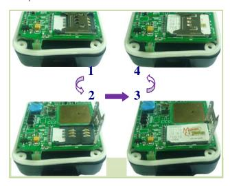
6.5. Switch on the tracker after inserting the SIM card into the tracker, and then you can enjoy your tracking time.
