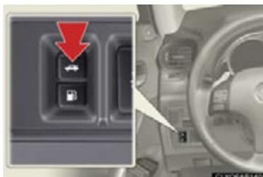
To open the trunk from inside the cabin, simply press the trunk opener.
