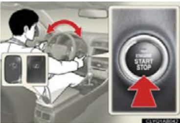
The steering wheel locks when the “ENGINE START STOP” switch is OFF and the driver’s door is opened.
