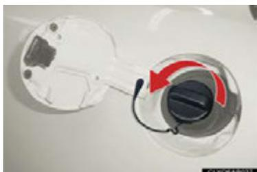
2 Slowly remove the cap by turning it counter-clockwise.
