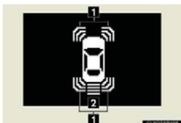
Sensors are used to detect obstacles near the vehicle. The distance to a detected obstacle is shown by the number of indicator bars.
