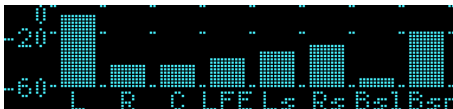
Figure 4-9 Level Meter Displaying a Dolby E 7.1 Input
