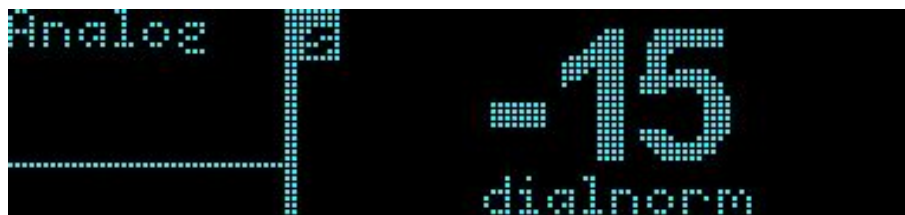
Figure 4-8 Main Status Screen Displaying a Recommended Dialnorm Setting for an Analog Input
