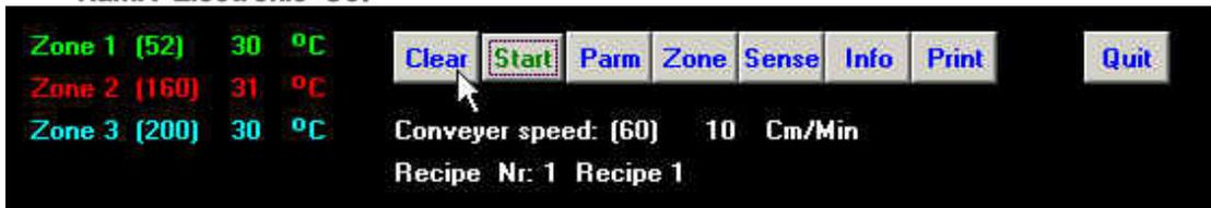
With the clear button you may clear the screen and the temperature measurement will start on the left side again.
