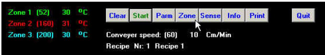
The zone button displays the temperature zone diagram, this is the diagram below.
