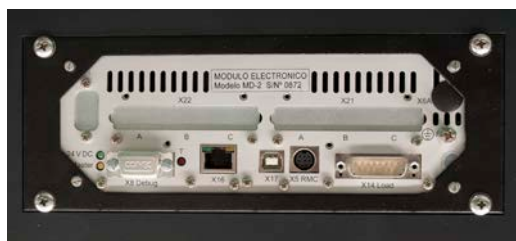
MD2 module, placed in the base housing of a TESTCOM machine
