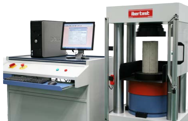
MEH LC 2000 MD2 W - with WinTest32 software and desktop PC computer
