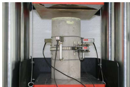
Compression elasticity of concrete. Young Modulus and Poisson Coefficient determination
