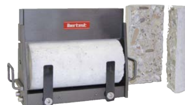
Indirect tensile (Brazilian test) as per EN 12390-6
