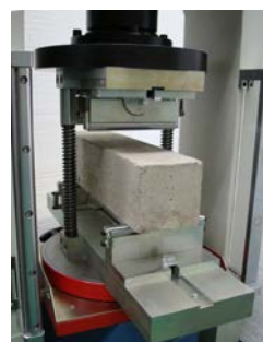
Flexural strength of concrete as per UNE-EN 12390-5
