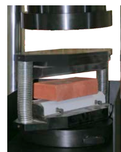
Indirect tensile of paver-bricks, as EN 1338
