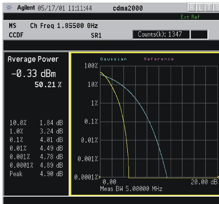
The CCDF measurement result should look like the above figure. The measurement result values are shown in the summary result window.
