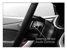
• Press the button in the center to select the next preset station (radio) or to change CDs if equipped with a CD Changer.
