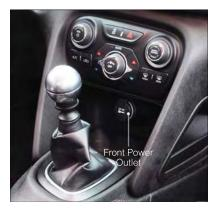
Power outlets are designed for accessory plugs only. Do not insert any other object in the power outlet as this will damage the outlet and blow the fuse. Improper use of the power outlet can cause damage not covered by your new vehicle warranty.
