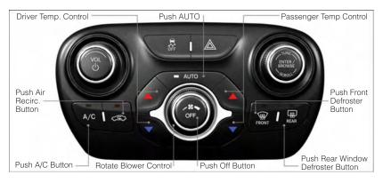
For your convenience the climate controls can be operated by using the soft-keys located on the touch screen or the climate control knobs below the Uconnect Touch<sup>™</sup> display.
