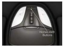
Erase all channels before you begin programming. To erase the channels, place the ignition switch into the ON/RUN position, then press and hold the two outside HomeLink<sup>®</sup> buttons (I and III) for up 20 seconds or until the red indicator flashes.
