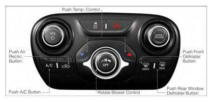
For your convenience the climate controls can be operated by using the soft-keys located on the touch screen or the climate control knobs below the Uconnect Touch™ display.
