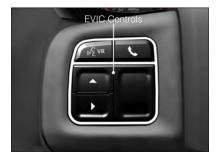
Press and release the SELECT > button to access the sub-menu screens of a main menu item. Press and hold the RIGHT arrow button for two seconds to reset displayed/ selected features that can be reset.
