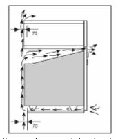
The unit panels next to the cooker must be heat resistant. In the case of veneered wood units, glues must be resistant to a temperature of 120°C.
