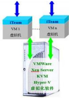
part indicates how iTeam works with VMs created by other virtualization software like VMware, XenServer, KVM, Hyper-V, etc.. Users only need to install iTeam into the Windows OS of the VMs. Nothing need to be changed to their virtualization platforms. See iTeam User Manual for more details.
