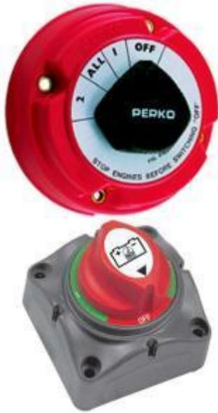
We do not recommend using an OFF – 1 – Both – 2 type battery switch,(as shown) this switch requires input from the skipper and if you forget to isolate your start battery you could run that flat overnight.
